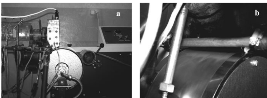
Figure 1 Film extrusion line (a), flow out from the flat die and compressed air-cooling of extruded material (b).
